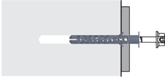
3] Insert MFA as through fixing
